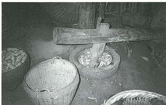
A Yu-Mien Yao woman pounding maize with a treadle-operated tilt-hammer pestle at Gulu Cun, Lina Cun Gongsuo, Dongpo Yaozu Xiang, Funing County, Yunnan, China.(雲南省富寧縣洞坡瑤族鄉里那村公所谷魯村) Orig.Photo: SHINTANI Tadahiko, 11 September 1991.)
