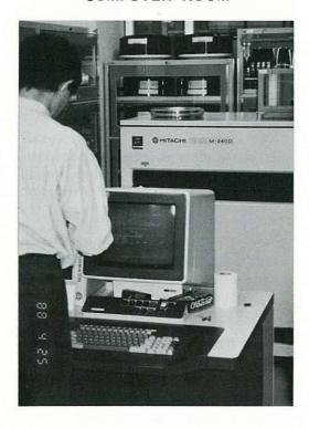
This room has housed the HITAC M-240D system since April 1983. The computer consists of a 12 MB memory, three disks of a total 5 GB, two optical disk units and three magnetic tape-decks.
