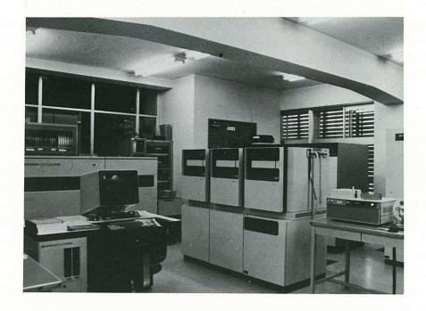
This room has housed the HITAC M-240D system since April 1983. The computer consists of a 12 MB memory, three discs of a total 5.4 GB and three magnetic tape-decks.
